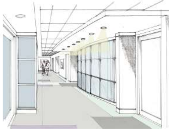
Corridor Rendering: Curved glazing at the Group Rooms introduces natural light deeper into the building.
